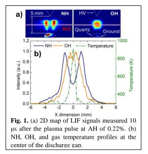
$N \rightarrow NH + O$  is the main pathway for NH formation. Meanwhile, the drop in NH intensity in the center of the plasma region is explained by temperaturepromoted NH removal through competitive processes, resulting in the formation of HNO, H<sub>2</sub>O, and NH<sub>2</sub>.
